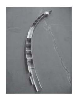
Laser-welded component. The part was originally machined from plate with a buy to fly ratio of 30:1. The laserwelded part shown had a buy-to-fly ratio of 3:1.
