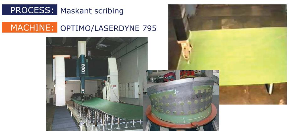
Process: cut through rubber maskant without damaging the base material (Al, Ti, Ni-alloys)
